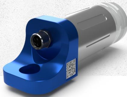
purePULSE is an easy to install long range wireless speed sensor made for contactless precise measurement of revolutions per minute. The speed sensors detect the motion of ferromagnetic structures, such as gearwheels or shafts, and in combination with pureMEMS it becomes the perfect tool for analysing applications with variable speed.
